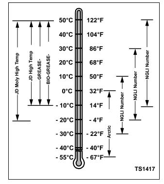
Use grease based on the expected air temperature range during the service interval.
